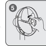
Place the blade onto the motor shaft, ensuring that grooves of the blade fit with the motor shaft pin. Place the blade cap over the blade and tighten it by twisting in the direction as shown by the arrow (TIGHTEN).
