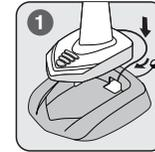
String the power supply cord through the hole in the fan base. Place the stand into the corresponding base slot and press on all sides. (Be careful not to let the power supply cord be squeezed between the fan and the base)
