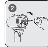
Loosen the blade cap by twisting it in the direction as shown by the arrow (LOOSEN).
