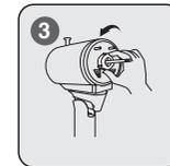
Loosen the back grille lock by twisting it in the direction as shown by the arrow (LOOSEN).
