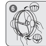
Assemble the front grille with the catch on the grille ring interlocking with the back grille clip lock. Press the grille ring in all directions then push the grille clip up.
