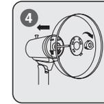
Assemble the back grille as shown in the diagram. Place the back grille lock over the grille and tighten it by twisting in the direction as shown by the arrow (TIGHTEN).
